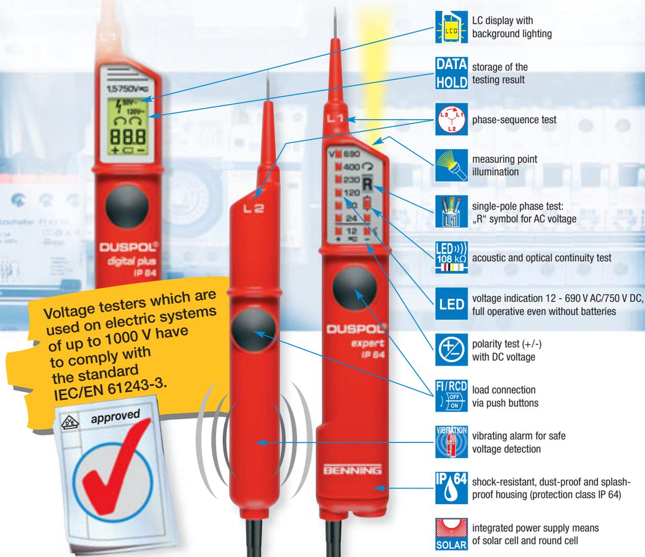
Voltage testers which are used on electric systems of up to 1000 V have to comply with the standard IEC/EN 61243-3.
