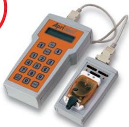
Customise Installer code and System code. Select access management functions. Select receiver output channel functions: pulse, hold, step-by-step and timer with 1-255 s programmable duration. Configure codes in memory modules or internal buffers. Configure remote controls with code customisation.
