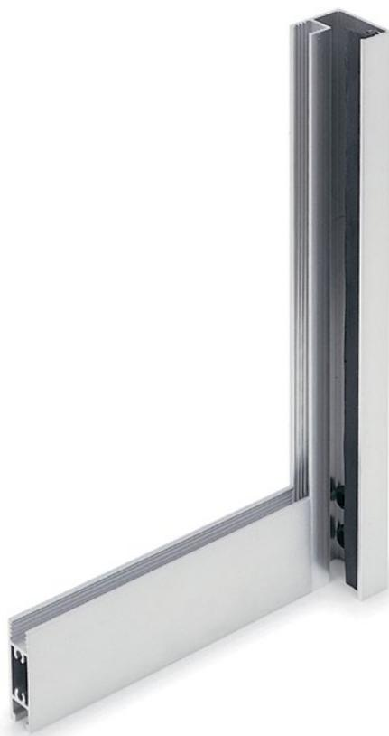
"SMALL" series profiles **can be used to make wings** for automatic sliding doors. This profile has been designed and manufactured specifically for mobile wings, fixed side wings and semi-fixed side wings. In spite of its compact size, the profile is compatible with up to 10 mm thick glass panels.
