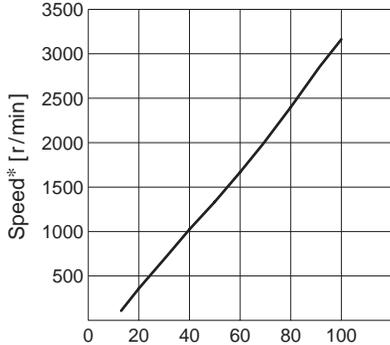
External potentiometer graduation – speed characteristics (typical value)
