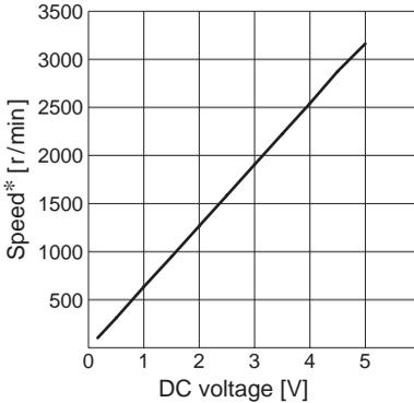
External DC voltage – speed characteristics
