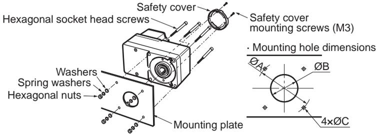
• Using the rear side as the mounting surface
