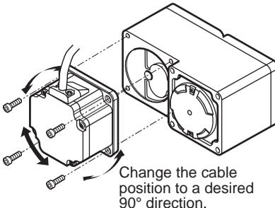
Change the cable position to a desired 90° direction.
