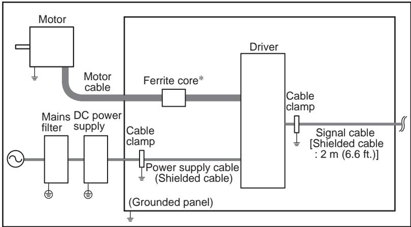
\* Use the ferrite core for extending the motor cable.
