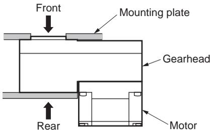
• Using the front side as the mounting surface
