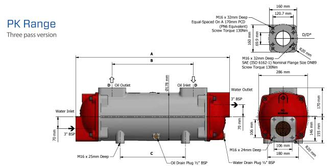
End Cover Screw Torque 130 Nm
