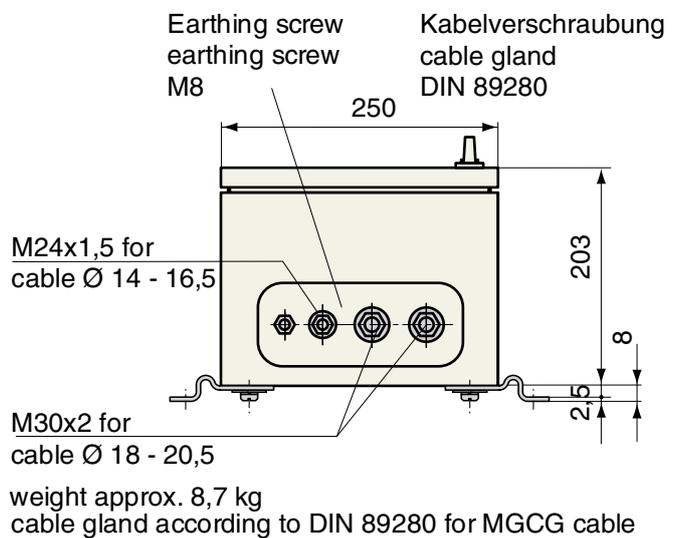
**Standard control box (supply voltage 380 / 440 V - control voltage 115 / 220 V) - other voltages on request**
