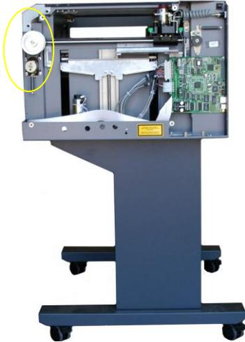
4. Get a feel for how tight the y-motor belt is by squeezing the sides. This will be used as a reference when tightening the belt back up after installing the new assembly.
