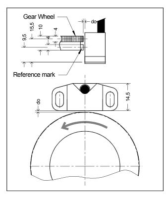
The arrow indicates the direction of movement during counter-clockwise rotation of the gear wheel with a view to the encoder
