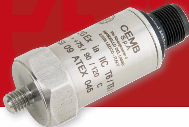
The integrated transmitter TR-26 measures the absolute vibrations of any rotating machine support and it is able to interface directly in 2 wires technique (current loop 4 ÷ 20 mA) to an acquisition system (PLC or DCS).
