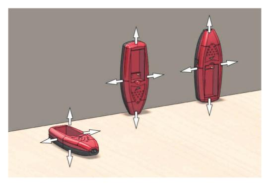
On the battery chargers back side there is four rubber knobs which secure a stable placing. There are also two mounting holes for wall mounting on the back side. It is recommended to use 4mm screws with head diameter of  $\emptyset$  5,5 – 7mm and head height of 1,5 – 2mm. Screw type and length need to be adapted to which material and thickness of the wall it shall be mounted on. See illustration pictures below.
