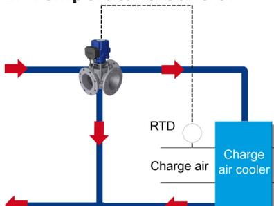
The intercooler is used to cool high temperature turbo charger air.
