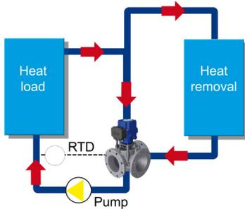
Lubricating oil temperature control is normally configured in a mixing application controlling the return temperature to the heat load. The temperature is normally measured as close as possible to the sump return.
