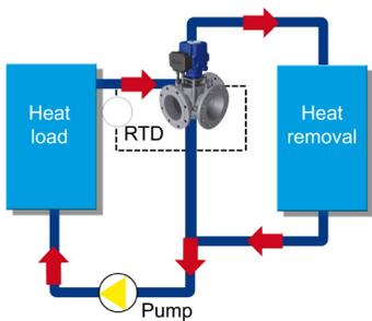
Jacket water cooling in diverting applications regulates the outlet coolant water temperature from a diesel or gas engine. The valve either sends water to a cooler or bypass loop, accurately maintaining the temperature.
