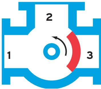
The unique construction of the AMOT G valve provides total flexibility by allowing you to select the valve port positions most ideally suited to meet your application requirements. There are two main types of mode of operation:
