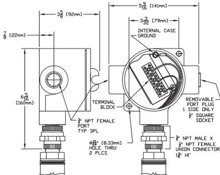
Junction box meets enclosure type 4 requirements only. Not ATEX compliant (see option M423 for ATEX junction box)
