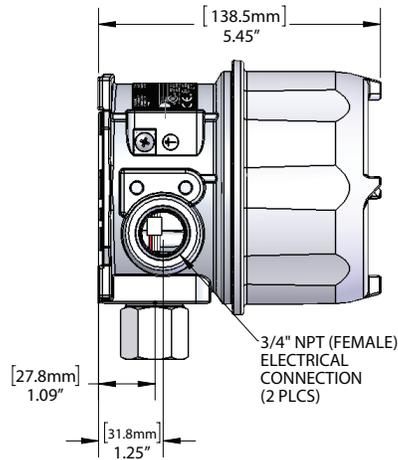
DISPLAY CAN BE ROTATED UP TO 180° BOTH DIRECTIONS
