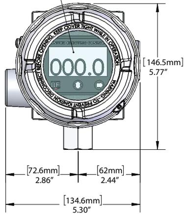
Shown with Dual Seal option M041 and gage pressure sensor
