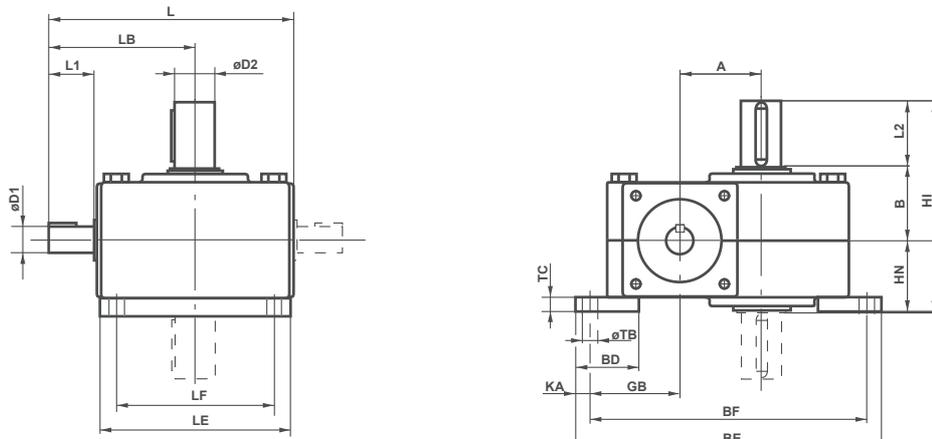
Mounting position HU, HN, HD. Also state position of input shaft
