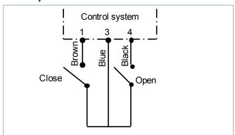
Computer, I.S. control or direct connected lamps or relays.
