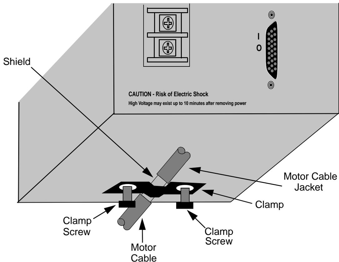
Figure 3-5: Terminating Incoming AC Power (Mains) Cable for 460V Drive
