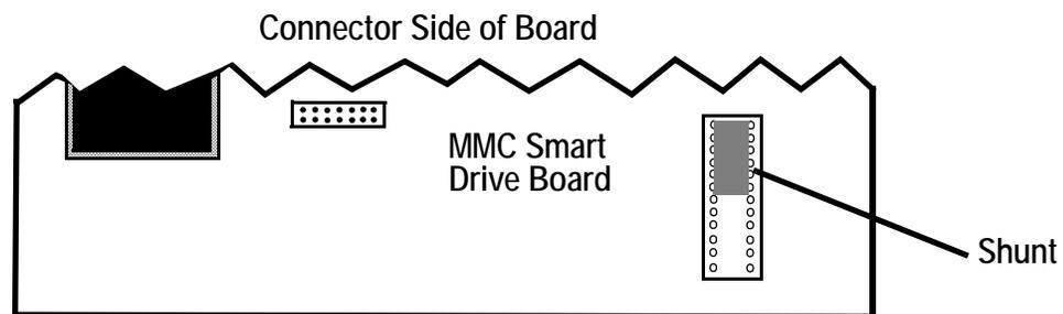
Figure 10-2: : Shunt Removed and Resolver Module Installed
