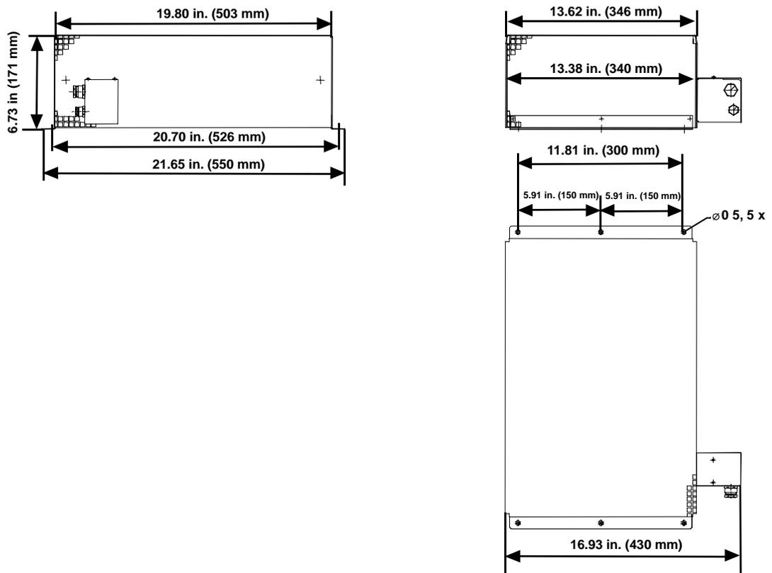
**Figure 4-7: Mounting Dimensions for 460V External Shunt (P/N M.1302.7063)**
