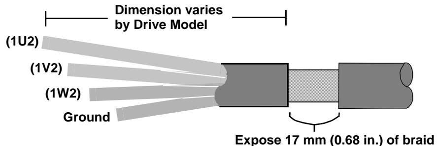
4. Attach the individual wires from the motor cable to their assigned terminal. Refer to Chapters 5 and 6 for front panel connectors and terminal assignments.
