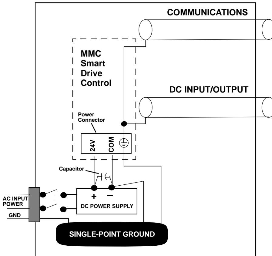
Inside a control cabinet, connect the shields of shielded cables. The two different methods of terminating shields are used to accommodate two different immunity requirements. Immunity required inside an enclosure is considered lower because cables are typically less than three meters in length and/or can be separated from each other and from noise sources.
