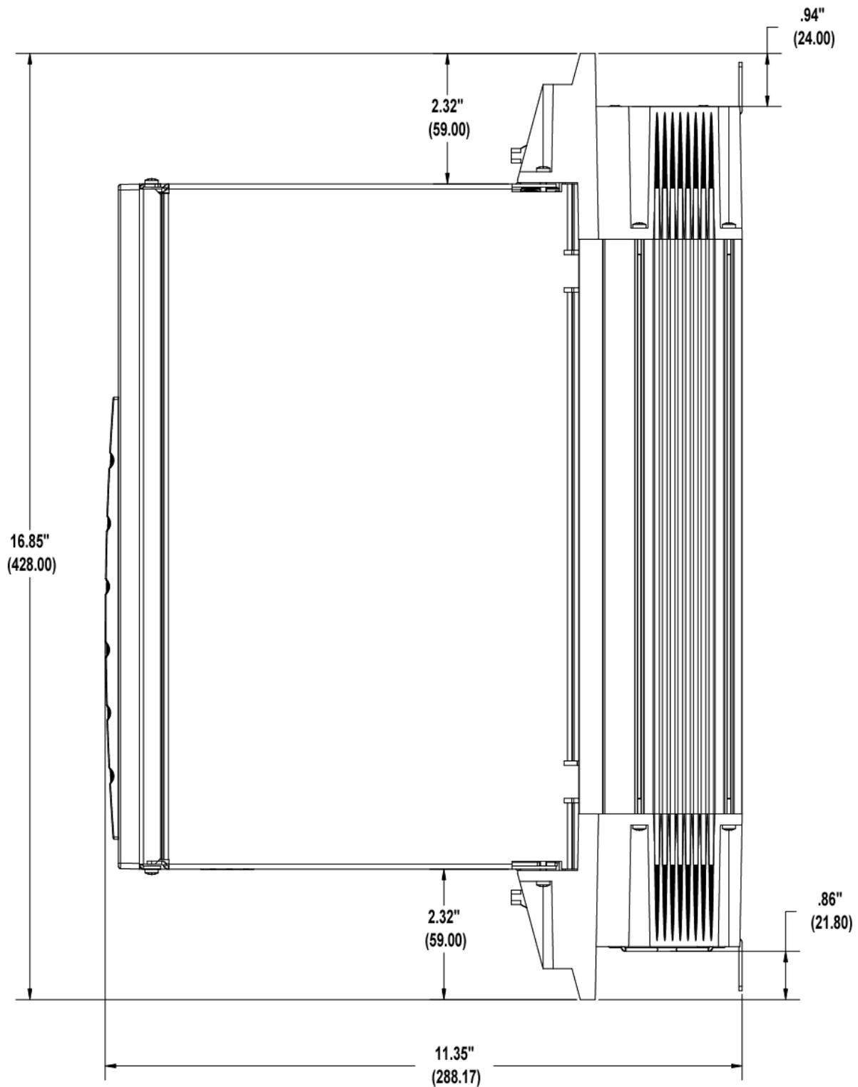
Figure 6-13: Size 3 460V Smart Drive - Front View
