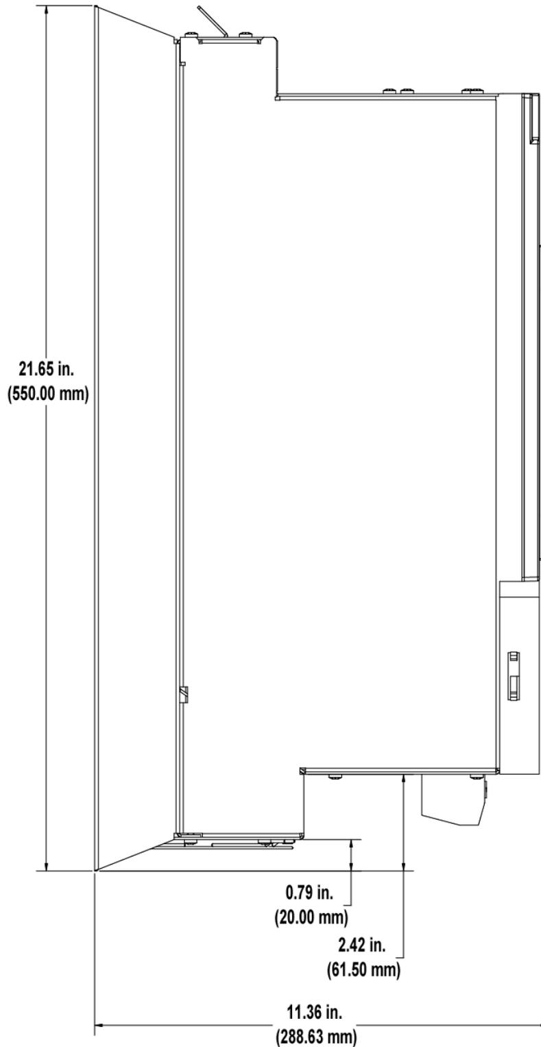
Figure 6-15: Size 4 460V Smart Drive - Front View
