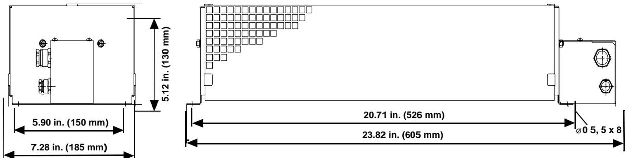
Figure 4-6: Mounting Dimensions for 460V External Shunt (P/N M.1302.7061)
