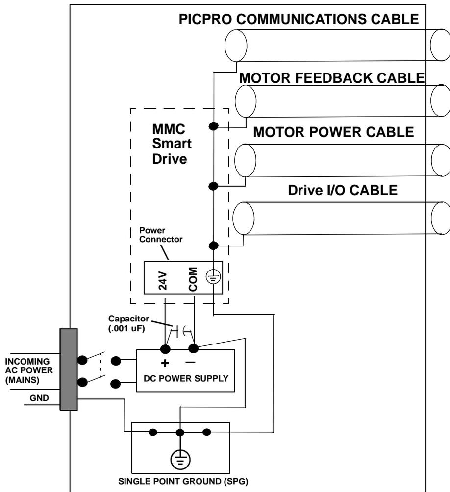
To prevent excessive conducted emissions from a DC power source (typically 24V) used for digital I/O, a .001 micro farad capacitor should be used. Connect the capacitor from the +24V DC to COMMON at the distribution terminals.
