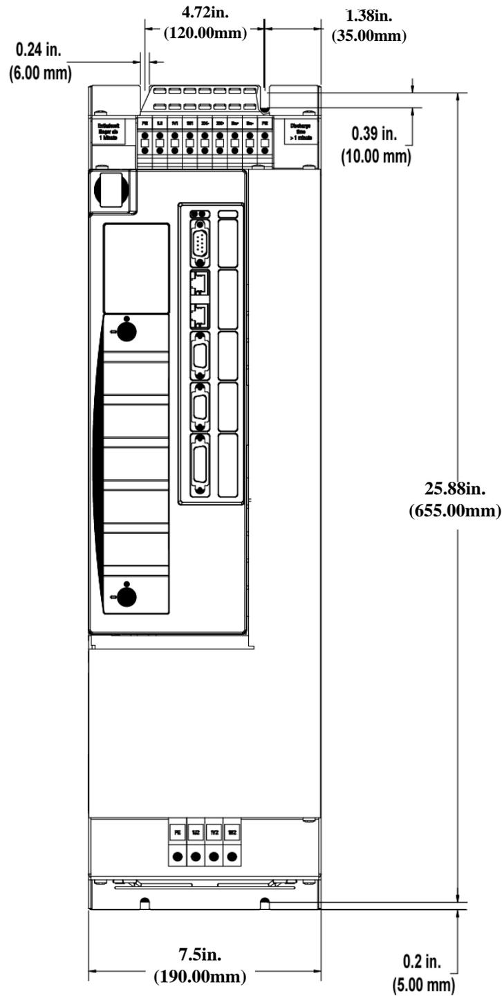
Figure 6-16: Size 4 460V Smart Drive - Side View
