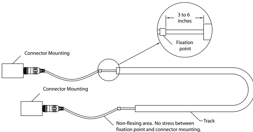
Observe the following precautions when installing flex cables:
