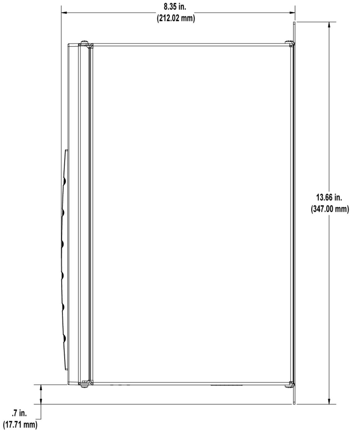
Figure 6-11: Size 2 460V Smart Drive - Front View
