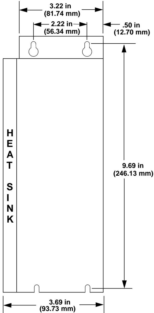
Figure 5-10: 1 kW & 2 kW Narrow Drive (-DN) - Front View
