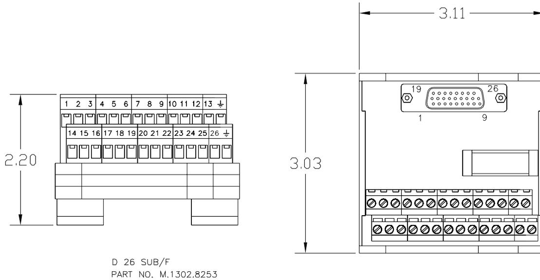
Figure 11-6: General I/O Port Breakout Board Dimensions
