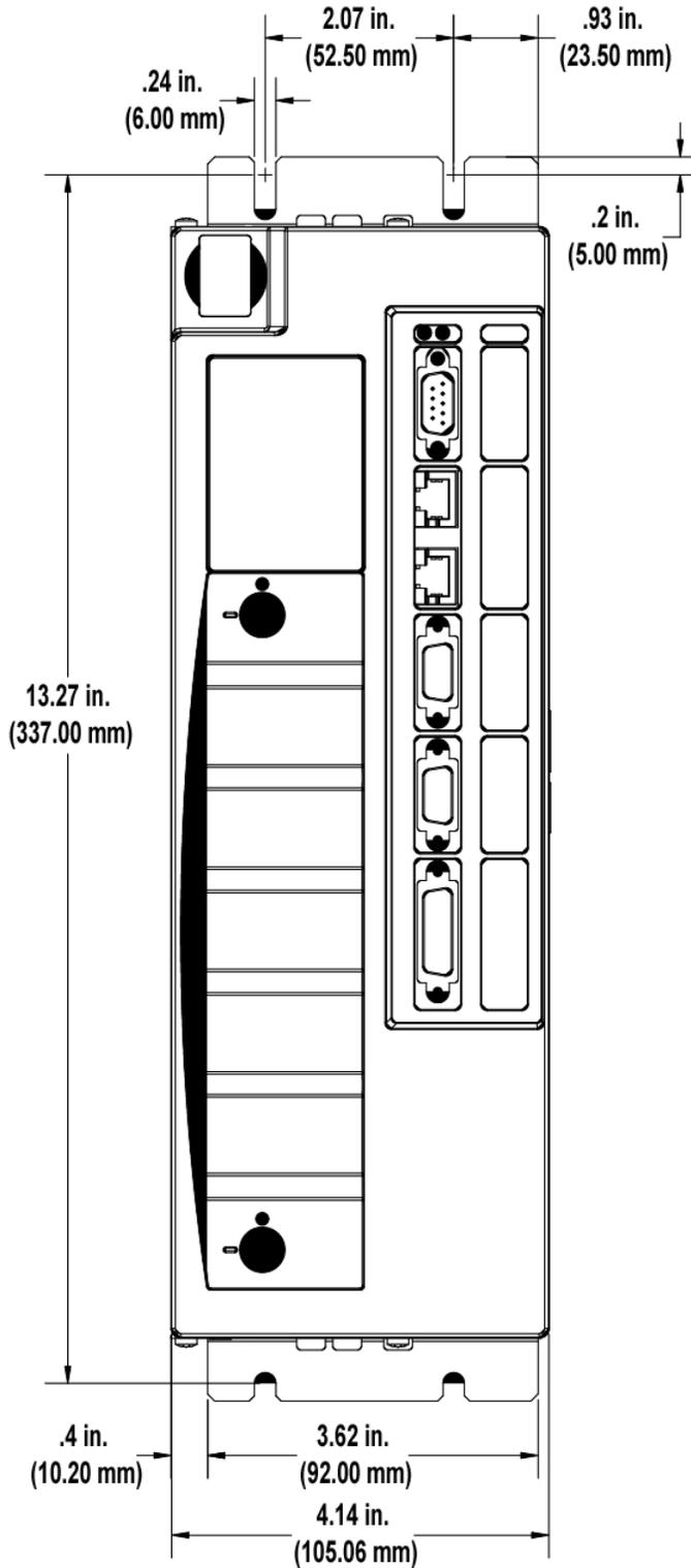
Figure 6-10: Size 1 460V Smart Drive - Side View
