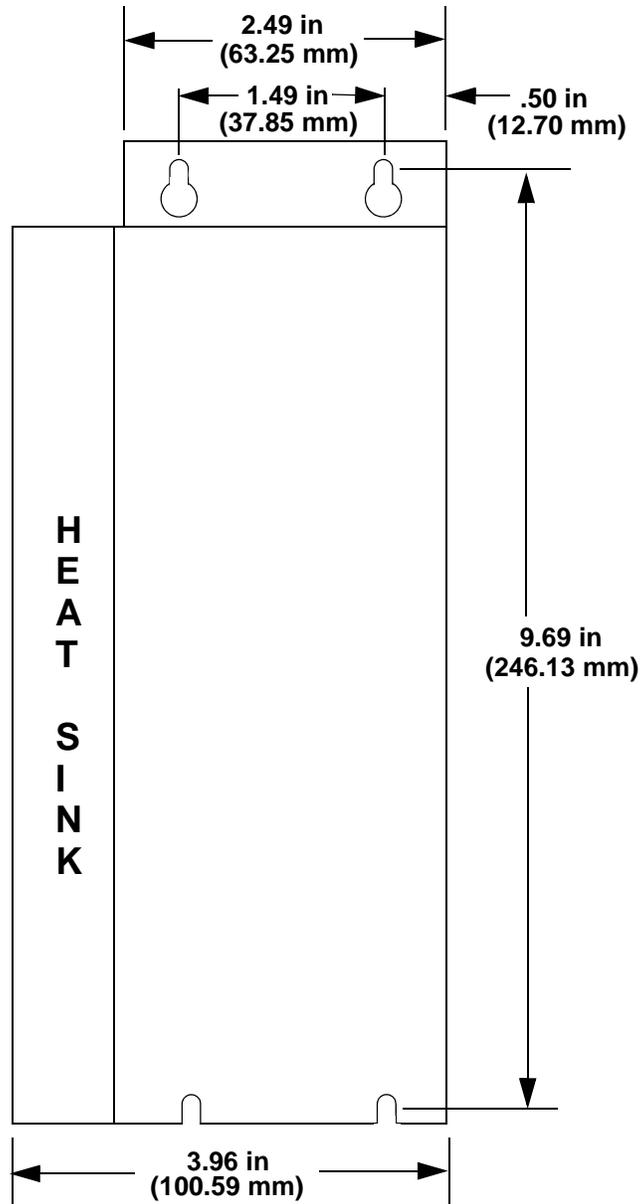
Figure 5-11: 1 kW & 2 kW Standard Drive (non-DN) - Front View
