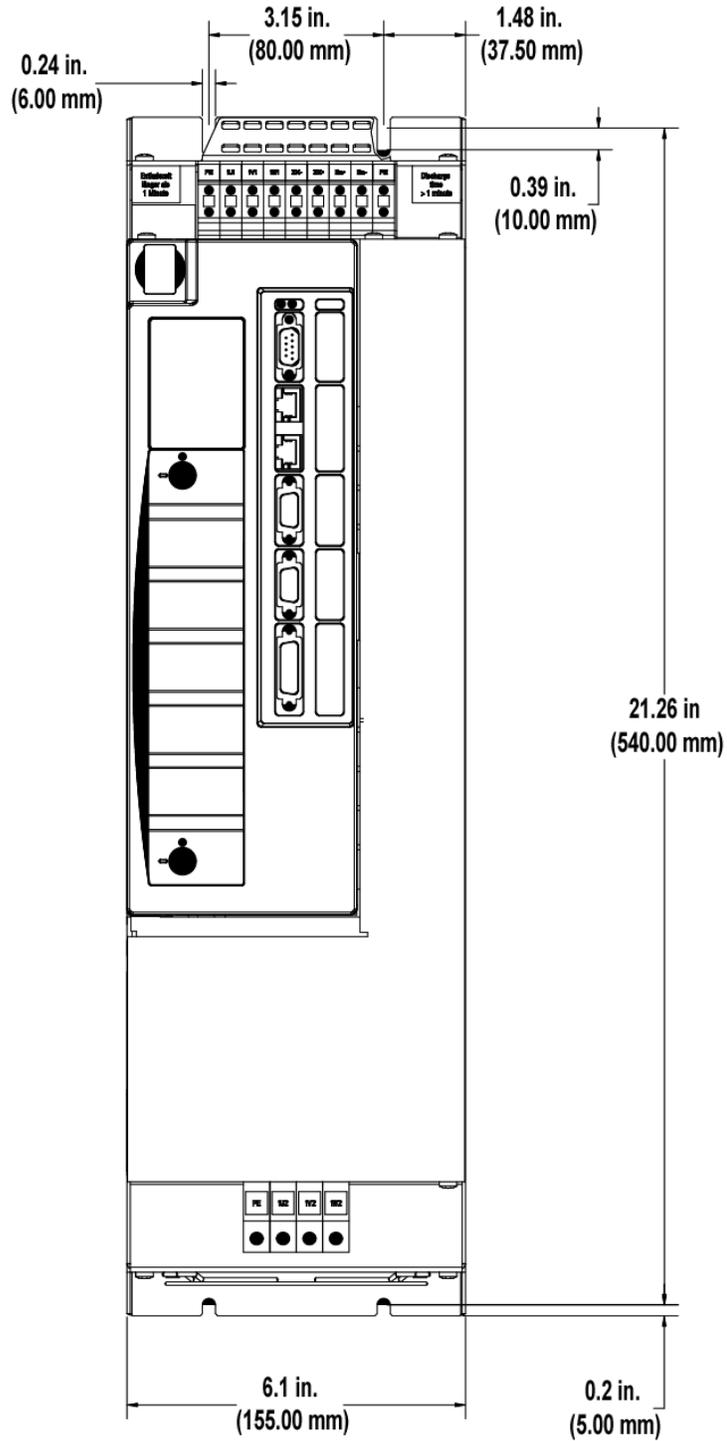
Figure 6-14: Size 3 460V Smart Drive - Side View
