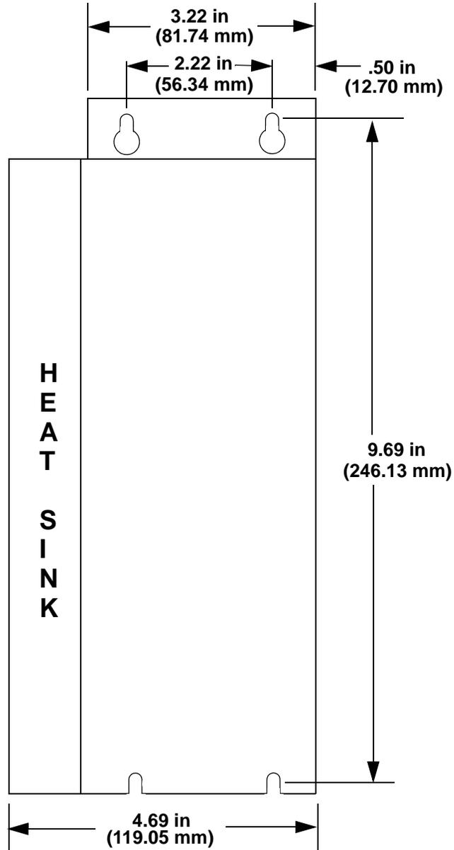
Figure 5-12: 230V Standard (non -DN) and Narrow (-DN) Drive - Side View
