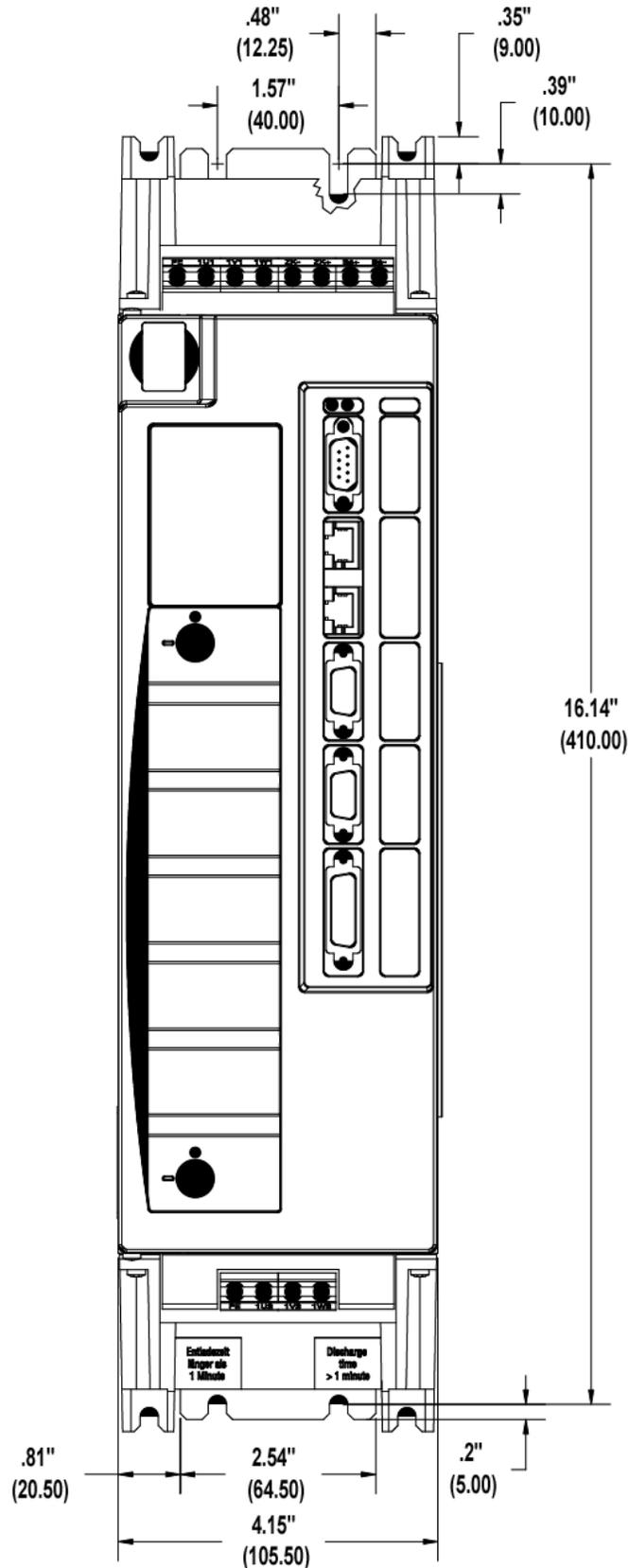
Figure 6-12: Size 2 460V Smart Drive - Side View
