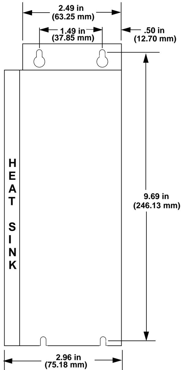
Figure 5-9: 500 W Standard Drive (non-DN) - Front
