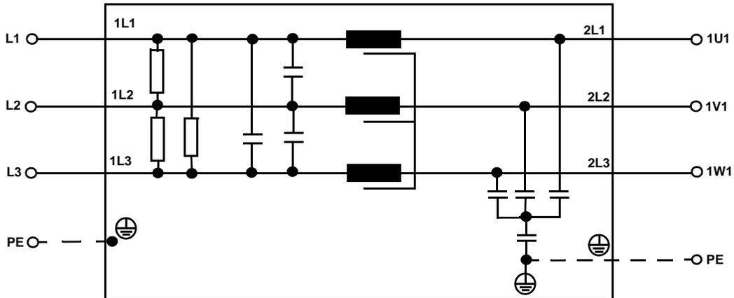
Figure 4-9: Connection Diagram for 3-Phase Line Filter
