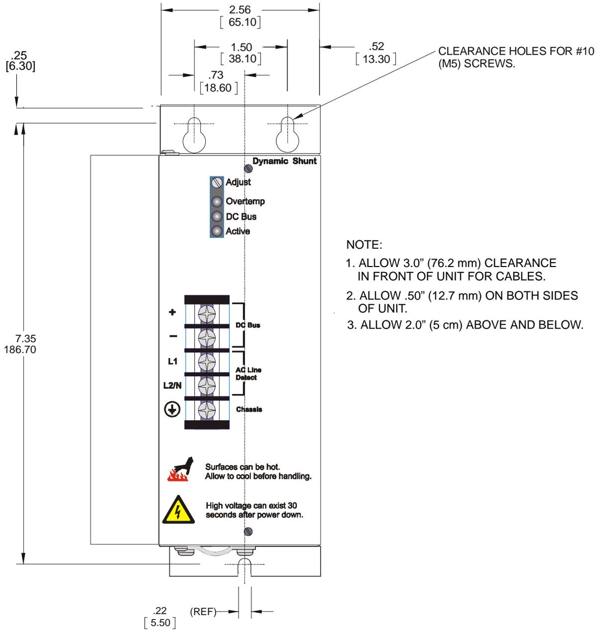
**Figure 4-3: Mounting Dimensions for 460V External Shunt (P/N M.1302.7048)**
