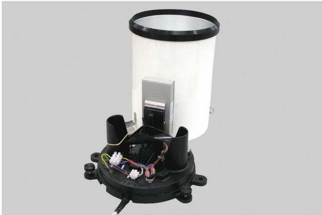
RG13H uses a pulse-based tipping-bucket mechanism to produce a contact closure every time it receives a predetermined small quantity of rainfall (0.1 mm / 0.004 in). RG13H provides accurate measurements. It is a robust system component that is suitable for remote and unattended locations.
