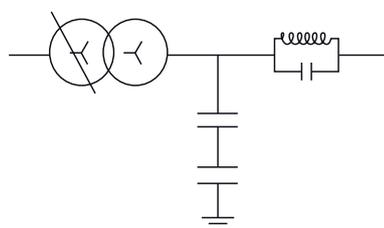
> 400 kV Capacitive voltage transformers. R.E.E. (Spain).
