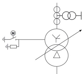
> 72.5 kV Combined transformers in substation incoming line. L'ONE (Morocco).
