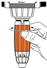
The injection rate is set by lining up the eyelet with the desired ratio on the scale. The amount of injected concentrate is proportional to the amount of water coming into the Dosatron: i.e. adjustment at 1% = 1 : 100 = 1 volume of concentrate + 100 volumes of water.
