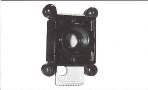
Arrow's new slide valve is a 3 way OSHA lockout valve which exhausts all downstream pressure when closed, and can be locked in the closed position with customer supplied padlock.
