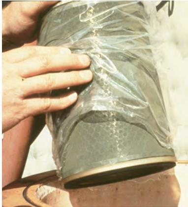
2. After removing the cartridge from the vessel, submerge it in clean fuel and gently scrub the entire screen surface with a soft bristle brush or a lint free cloth.
