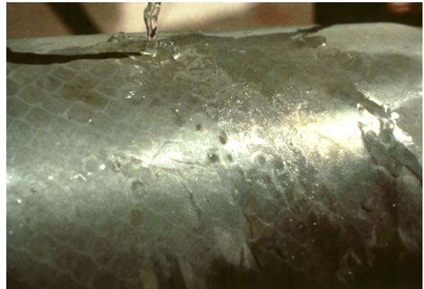
6. If any portion of the PTFE coated screen is wetted by the water (the water will seep into the pores of the screen; this is very obvious to the eye), the cartridge has failed the Water Test. The wetted area must be cleaned again (see Step 7), and the recleaned cartridge should pass the Water Test before it is reinstalled.
