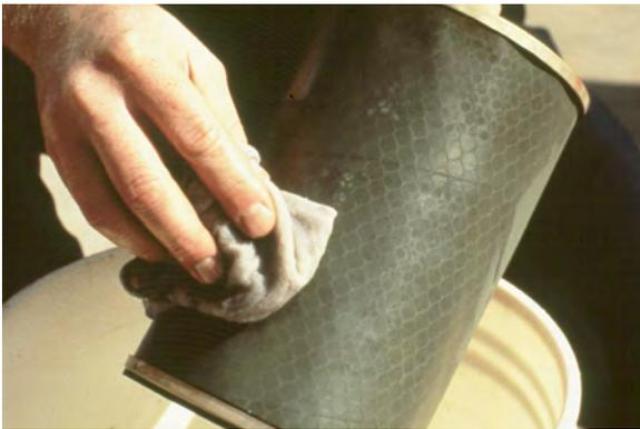
3. **SURFACE INSPECTION.** Holding the cartridge by the endcaps, visually inspect the entire surface of the screen for any nicks or cuts. If there are any visible flaws, they should be patched (see Step 6).
