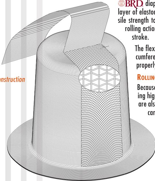
Fig. 2: BRD Construction
