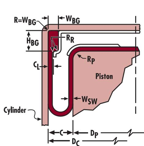
Fig. 32: Axial Compression with Stamped Retainer Plate
