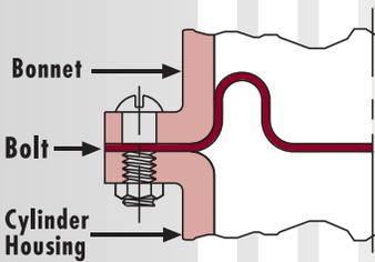
Fig. 23: Bolted Flange
