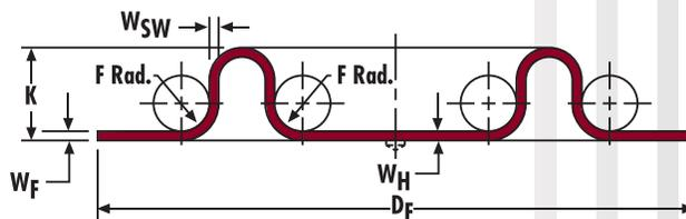
Fig. 10: Preconvoluted Diaphragm
