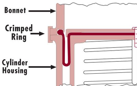
Fig. 29: Crimped Ring
