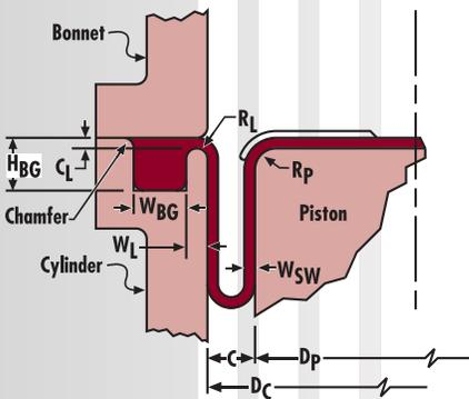
Fig. 24: Classes 3 and 3C Hardware Dimensions
