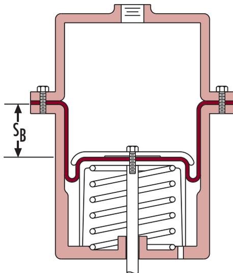
Fig. 6: Down-Stroke Position
