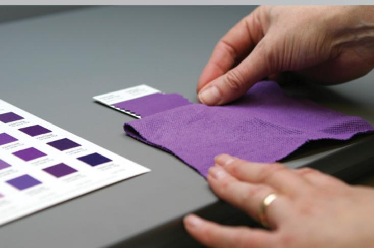
Colour requirements for manufacture and retail are complex and diverse. To ensure product colour, several types of light source are used (e.g. Artificial Daylight and a Point of Sale Light). Multiple light sources are also necessary to reveal colour inconsistencies and metamerism.
