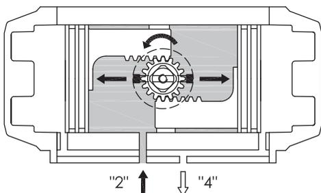
Air supplied to port 2 forces the pistons towards the actuator end caps. A counter-clockwise rotation is achieved. Exhaust air exits from Port 4.
