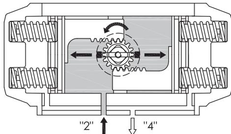
Air supplied to Port "2" forces the pistons toward the actuator end caps, compressing the springs. A counter-clockwise rotation is achieved. Exhaust air exits from Port 4.
