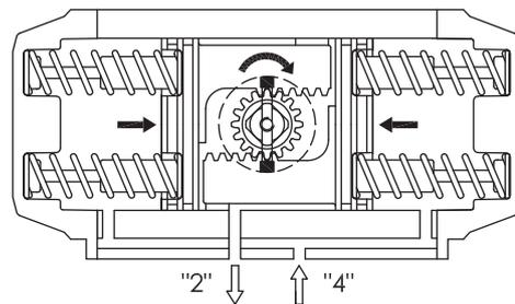
The loss of air pressure (air or electric failure) at Port "2" allows the springs to force the pistons inward. A clockwise rotation is achieved. Exhaust air exits from Port 2.
