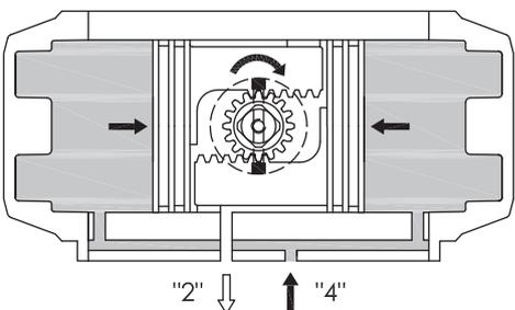
Air supplied to Port 4 forces the pistons inward. A clockwise rotation is achieved. Exhaust air exits from Port 2.
