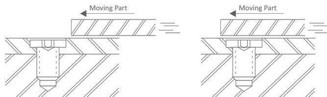
High Strength Fasteners for applications with limited clearance.
