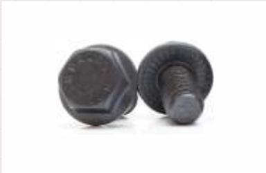
Durlok free spinning self-locking bolts are designed with long, ramp shaped, radial teeth blended evenly into a smooth slightly conical outer surface. Reusable. Self-locking. Anti-vibration.
