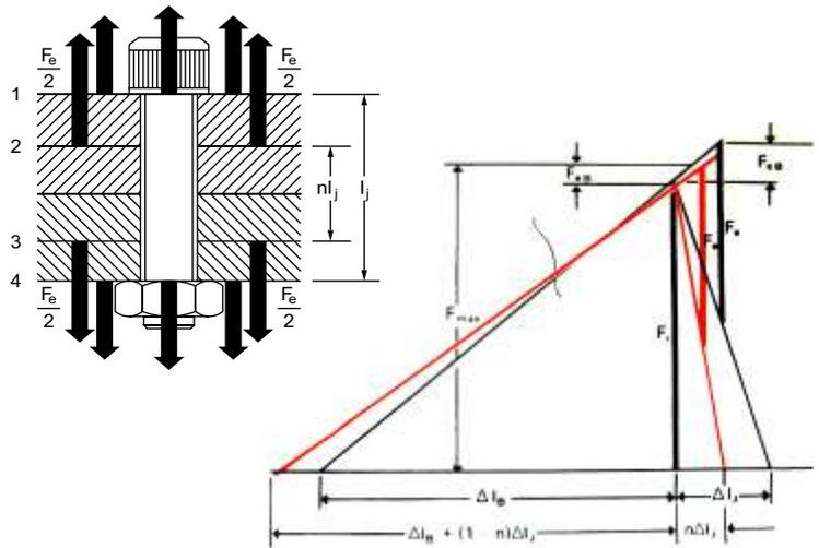
**Fig. 8 Joint diagram shows effect of loading planes of  $F_e$  on bolt loads  $F_{eB}$  and  $F_{B \max}$ . Black diagram shows  $F_{eB}$  and  $F_{B \max}$  resulting from  $F_e$  applied in planes 1 and 4. Orange diagram shows reduced bolt loads when  $F_e$  is applied in planes 2 and 3.**
