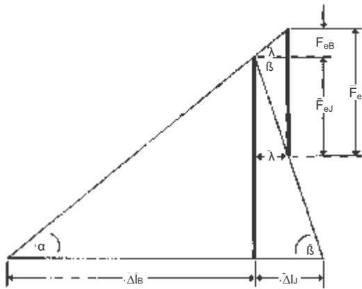
**Fig. 7 Analysis of external load  $F_e$  and derivation of Force Ratio  $\Phi$ .**
