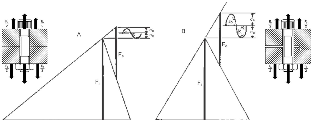
**Fig. 6** Joint diagram of a springy bolt in a stiff joint (A), is compared to a diagram of a stiff bolt in a springy joint (B). Preload  $F_i$  and external load  $F_e$  are the same but diagrams show that alternating bolt stresses are significantly lower with a springy bolt in a stiff joint.
