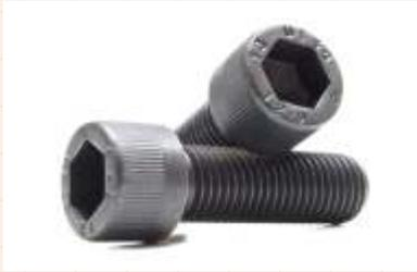
Suitable for all high tensile applications. Up to 1300 Mpa– highest of any socket cap screw. Use Stainless for corrosive, cryogenic or elevated temperature environments.
