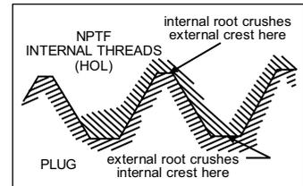
**PTF fully formed Dryseal threads** designed to achieve seal in tapped holes without need for sealing compounds.
