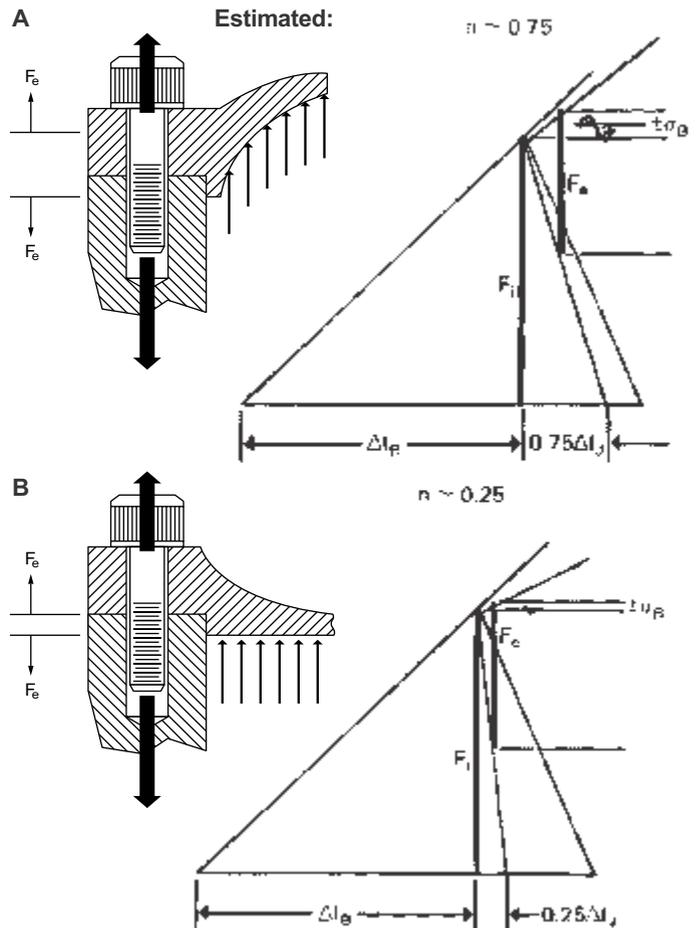
**Fig. 9 When external load is applied relatively near bolt head, joint diagram shows resulting alternating stress  $\alpha_B$  (A). When same value external load is applied relatively near joint center, lower alternating stress results (B).**
