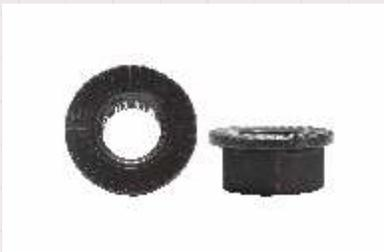
Durlok nuts are designed with long, ramp shaped, radial teeth blended evenly into a smooth slightly conical outer surface. For use with Durlok Bolts. Self-locking. Anti-vibration. Reusable.
