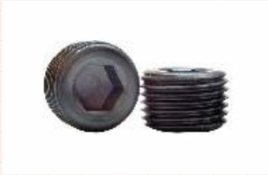
Levl-seal features: controlled 7/8" taper in 3/4" taper hole seats plug level, flush with surface within 1/2 pitch.
