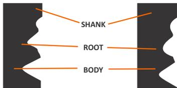
**CONVENTIONAL THREAD RUNOUT** - Note sharp angle at root where high stress concentration soon develops crack which penetrates into body of the screw.
