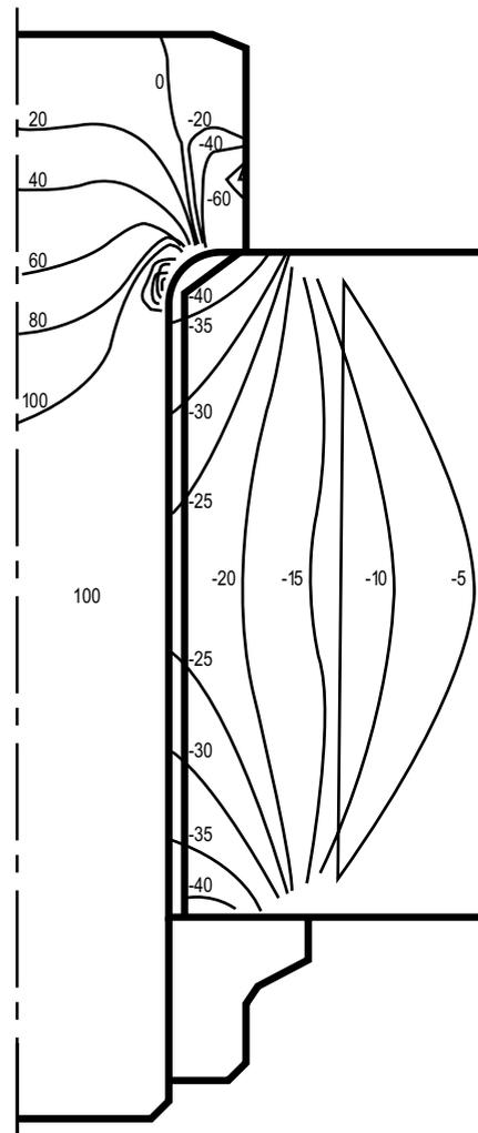
**Fig. 5 Lines of equal axial stresses in a bolted joint** obtained by the axisymmetric finite element method are shown for a 9/16—18 bolt preloaded to 100 KSI. Positive numbers are tensile stresses in KSI; negative numbers are compressive stresses in KSI.
