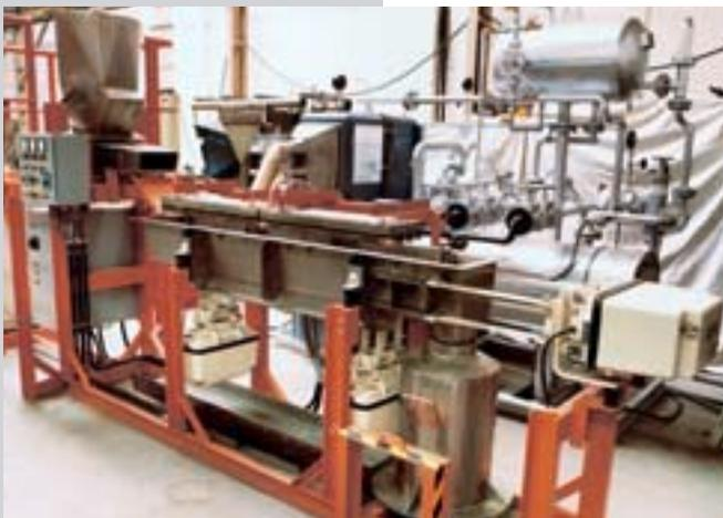
In the vibration fluidised bed, plastic granulate, for example, passes over a microsieve. Hot air dries precisely to the specified remaining moisture content. A close-loop control circuit regulates the speed of flow in dependence on the degree of drying, using simply voltage control on the drives
