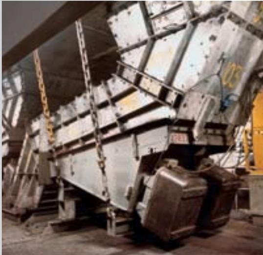
Vibrating tables with continuously adjustable magnetic vibrators ensure perfect material compaction in production and during packing
