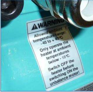
With an unbalance motor that is equipped with a standstill heater you should find the following label on the housing of the drive.
