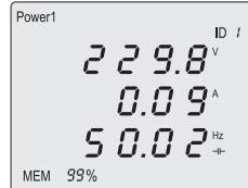
The maximum and minimum values are saved by the measuring device automatically. Via the „max“ (4) or „min“ (3) keys, the values are displayed for approx. 10 seconds. Pressing the key again switches back to the normal display prematurely.
