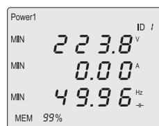
→ In order to delete the MAX/MIN memory, keep the two „min“ and „max“ pressed simultaneously for approx. 2 seconds. The data is deleted if „MAX/MIN“ appears on the display simultaneously.
