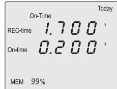
Via the two arrow keys (3 and 4) the days can be browsed back and forwards. This is illustrated under the display masking „Today“, e.g. as „1“ to „9“. After the „9“ display, the entire time (total) is displayed.
