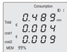
By pressing the „MODE“ key for at least 3 seconds, all displays of „Consumption“, „History“, „ON time“ and „Forecast“ are reset to null, and the „MEM“ memory deleted.
