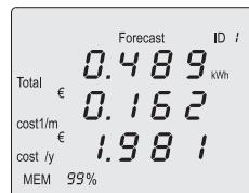
→ The already used energy (total in kWh) is used as the basis of the calculation. This calculated value is only an idea which represents the possible cause. Short measurement brakes or changed power prices can result in deviations. The measurement device is not approved for balancing purposes.
