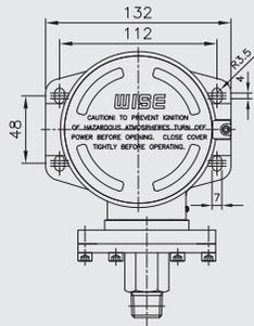
②-1 Nominal diameter  $\phi 88$  ( $\phi 98$ ) : 7.5 ~ 50 kPa (Pmax. 10 bar)
