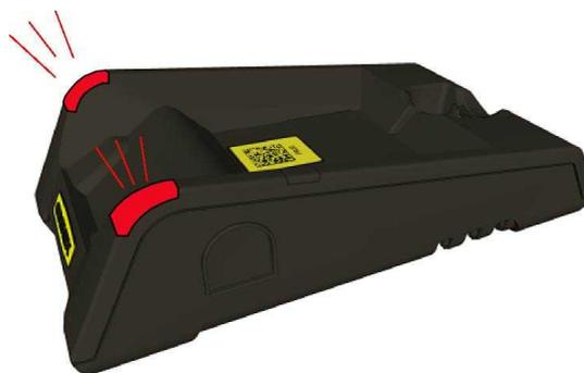
The base station that is paired with a certain reader signals a bad reader alert (beeps and flashing red indicators) also when another, unassigned reader is put into it.
