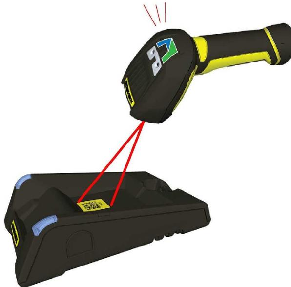
**Note:** Scanning the Pair code puts the base station and the reader put on it into **force pairing mode**. This means that the reader and the base it is put on get paired regardless of any assignments they both had previously. This force pairing mode is valid for 20 seconds after reading the Pair code.
