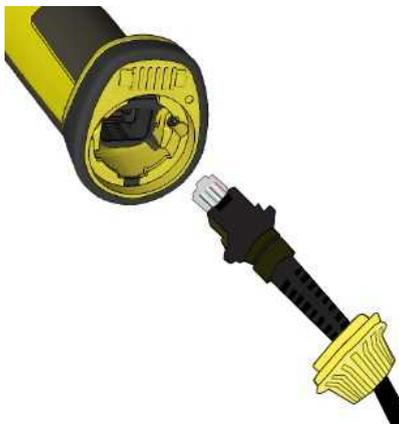
Use the DM8500-USB-00 cable (2.5 meters) or the DM8500-USBC-02 cable (2.5 meters).
