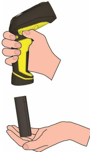
**CAUTION:** The battery used in these devices may present a risk of fire or chemical burn if mistreated. Do not disassemble, heat above 60°C (140°F), or incinerate. Replace battery with Cognex DMA-HHBATTERY-01 only. The use of another battery may present a risk of fire or explosion.
