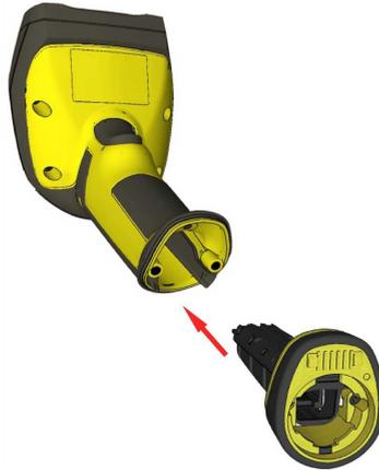
2. With a 2.5 mm Allen wrench, tighten the screws so that the side-in is firmly locked.
