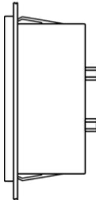
Fastening according to DIN 43 835 With screw clamp, panel thickness 1 mm to 4 mm (standard type, Figure 1) with DIN screw clamp shape B, panel thickness 1 mm to 40 mm for types 72 DIN, 96 DIN, 144 DIN (Figure 2) against surcharge
