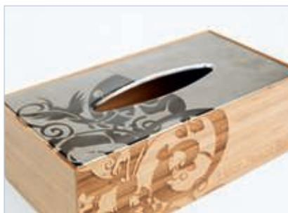
CO<sub>2</sub> laser for engraving wood, fiber laser for marking metals
