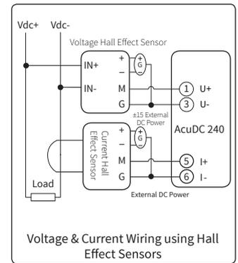
**NOTE:** Hall effect sensor can also be powered using the ±15V power supply from the X5 module.
