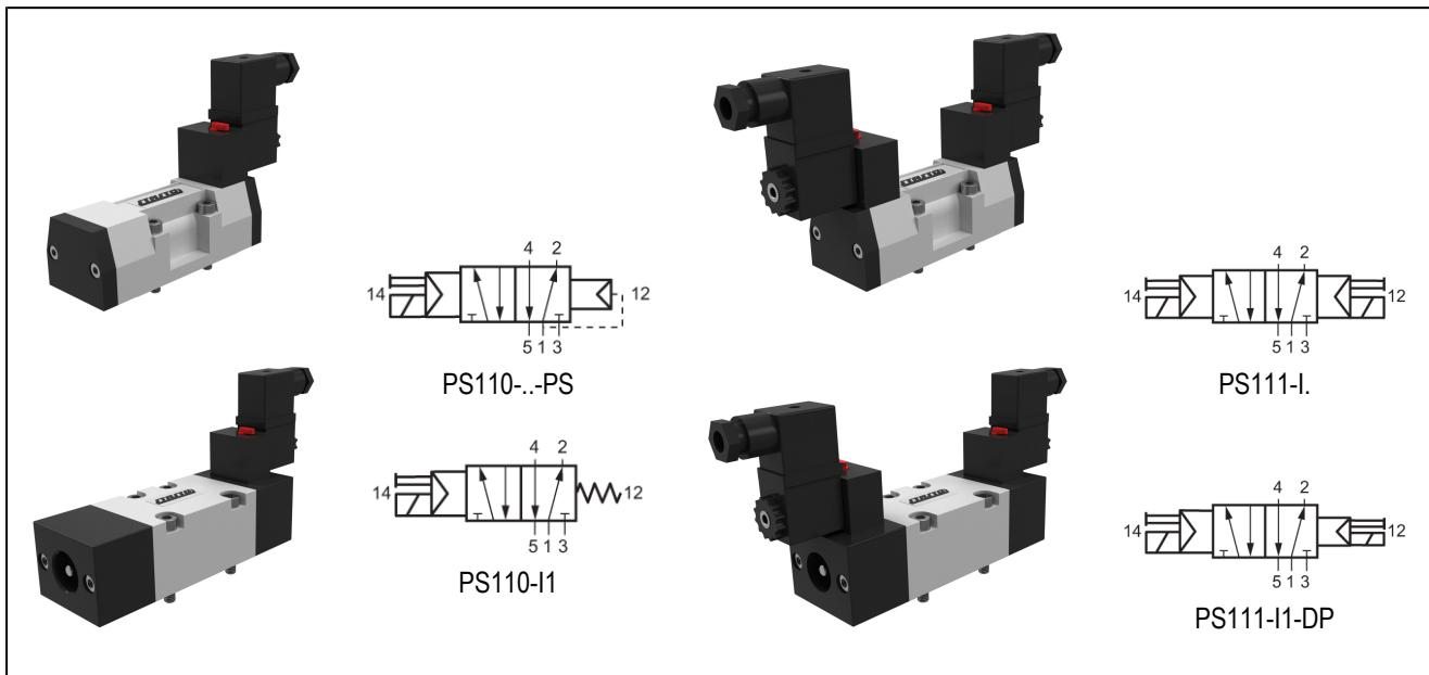
**design** 5/2-way solenoid valve pilot-operated, actuation electrical/internal control air, electrical/spring, electrical/electrical respectively electrical differential, manual emergency override, according to ISO 5599/1 size ISO1 and ISO2
