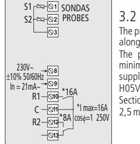
The probe and its lead should NEVER be installed in ducting along with power, control or power supply wiring.
