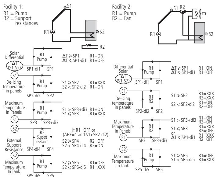
If E1 (Sensor 1 Failure) R1 = ON, R2 = OFF      If E1 (Sensor 1 Failure) R1 = ON, R2 = ON
