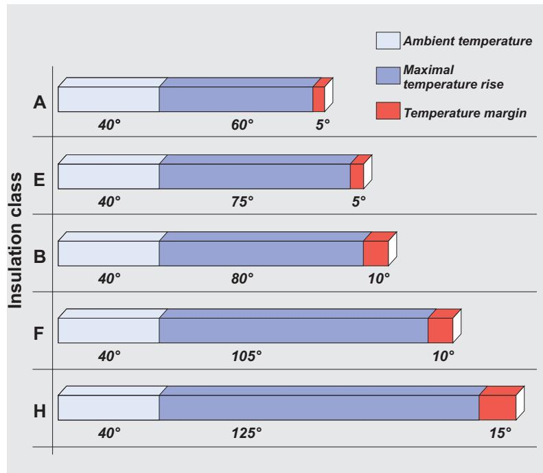
*Insulation class F in an electric motor means that at ambient temperature of 40°C the temperature rise of the winding may be max. 105°C with the additional temperature margin of 10°C (under specified measuring conditions in accordance with the IEC 60034-1 standard).*
