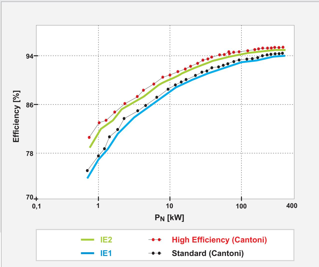
The efficiency class system specified under IEC 60034-30 is valid for low voltage three phase squirrel cage induction motors with the following specifications:
