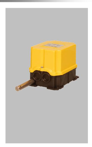
The rotary limit switch is a device which allows you to control the movement of industrial and building machines. The shaft is connected to the motor, so that, after a certain number of turns, the cams make the switches work, and then they can carry out their pre-set manoeuvre.
