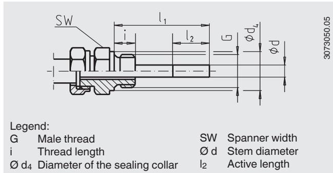
**Option:** Connection with union nut M24 x 1.5 and loose threaded connection M18 x 1.5
