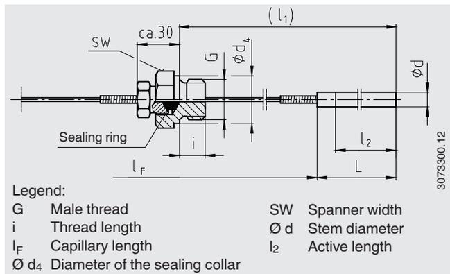
For stem diameter 6 mm no bend protection spring will be fitted at the probe.
