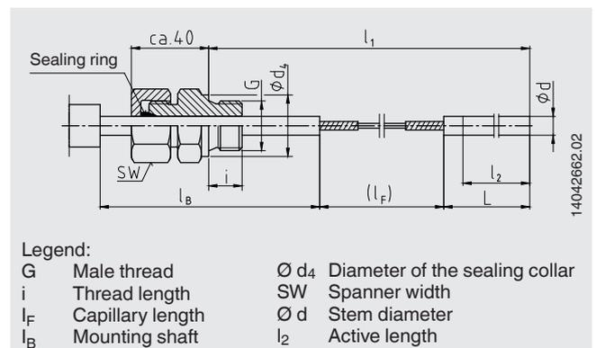
For stem diameter 6 mm no bend protection spring will be fitted at the probe.
