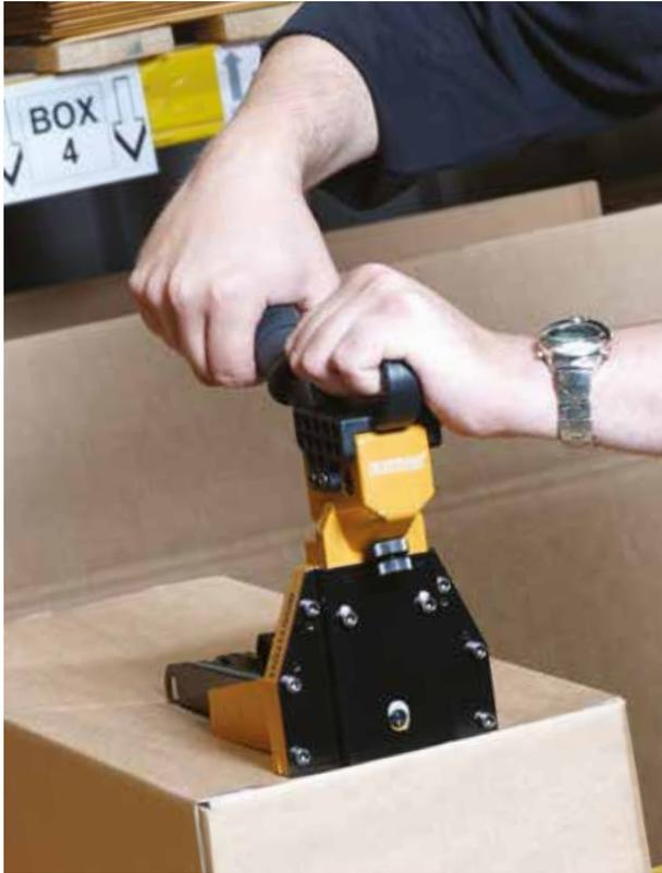
Fitted with a comfortable to use top grip and made from rugged aluminium, these manually operated tools are ideal for lower volumes of top sealing for single and double wall cartons.
