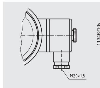
**B** Junction box made of PA 6, black, ingress protection IP65
