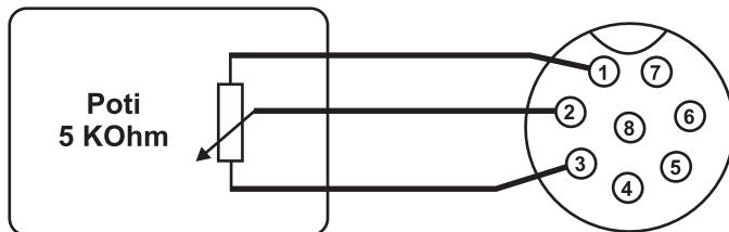
Switch off the switched-mode power supply and then connect the REMOTE plug to the rear remote connection. Screw the external fastening ring.
