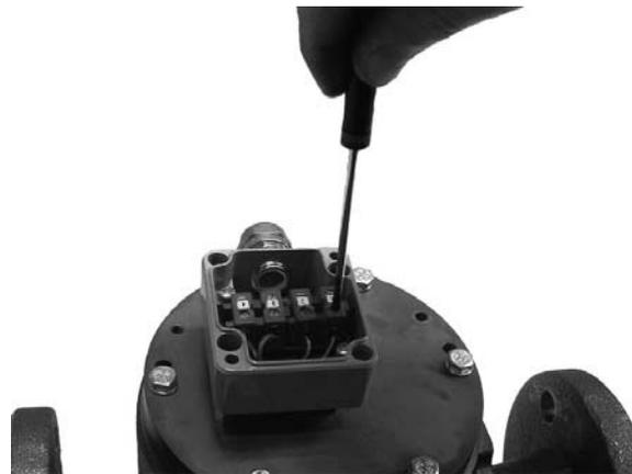
Disconnect the wiring (external and internal connections), pulse - red, temperature - green. Please make sure to write down how the connections are made.
