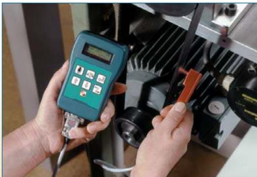
The BTM-400PLUS's LED-optical sensor is unaffected by ambient noise, offering improved performance versus competitive, acoustic sensor-based designs
