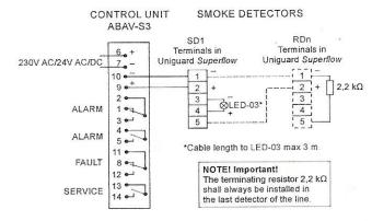
The alarm relay and the failure relay outputs are shown in alarm/no power on condition and the service alarm relay is shown in operative/no power on condition.
