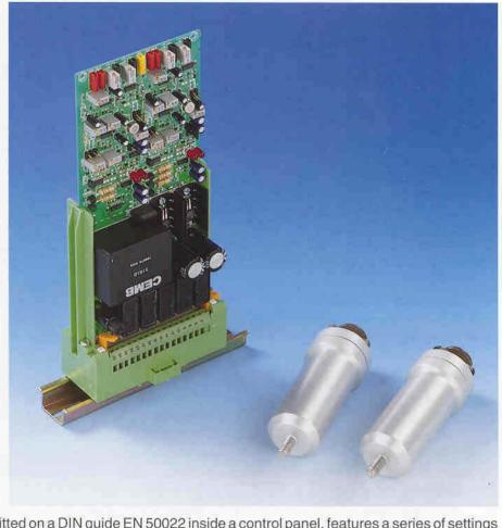
The processing module, which can be fitted on a DIN guide EN 50022 inside a control panel, features a series of settings which can be made by the customer for selecting optimum measuring parameters, delay time for the alarms, scale range, etc. The module is implemented with SMD technology to compact size and improve reliability.
