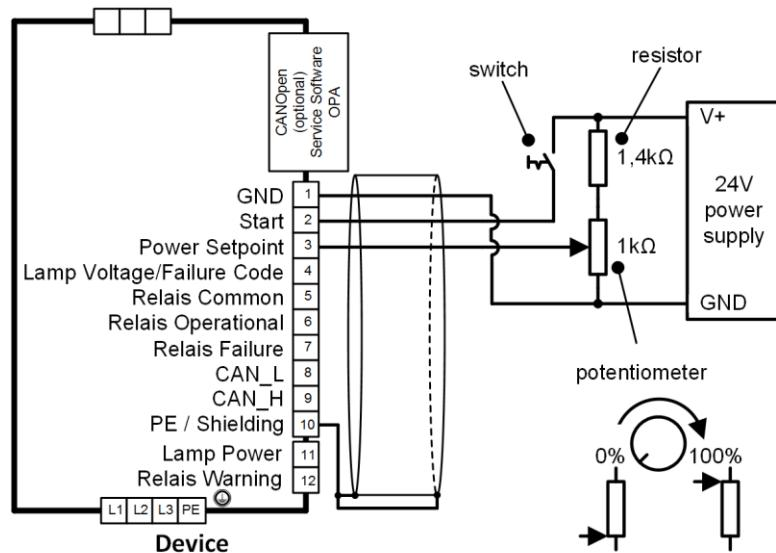
**SAMPLE CONNECTION OF ANALOG PLC CONNECTION**
