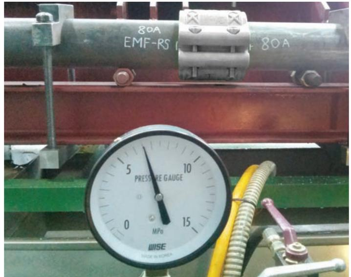
80A 6.5Mpa (65kg/cm<sup>2</sup>) Pressure Test
