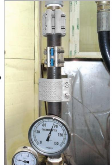
80°C x 30min. x 20kg/cm<sup>2</sup> High-temperature circulation test
