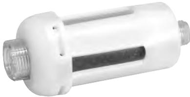
Used at the point-of-use, this disposable, mini inline desiccant dryer removes all traces of water vapor, oil vapor and dirt. It is often used directly upstream of blow guns or spray guns as final protection for critical parts blow off and paint spraying. Install in either direction; it functions in both directions.
