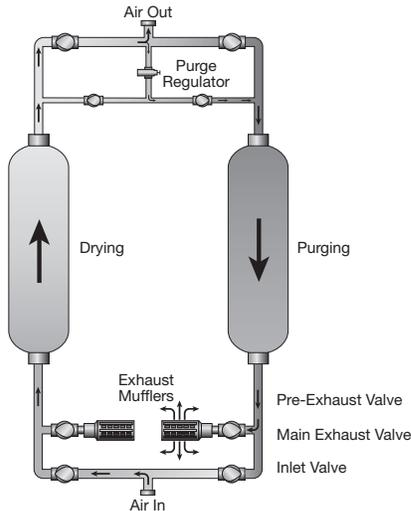
As the saturated compressed air flows up through the “on line” tower, its moisture content adheres to the surface of the desiccant. The dry compressed air is then discharged from the chamber into the distribution system.
