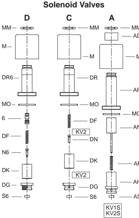
In case of down leakage, replace and test in the following order:
