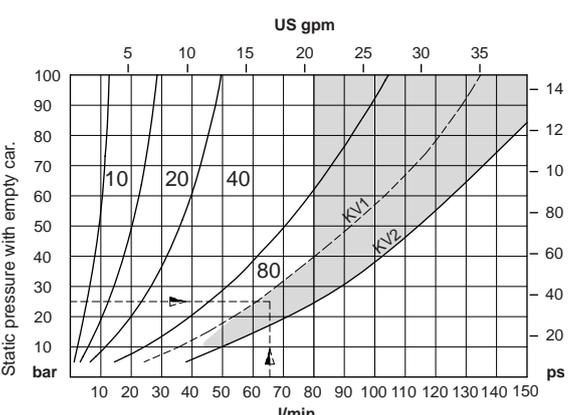
For pressure-flow conditions within shaded area, use 3/4" piping to avoid unnecessary power loss. Pump flows above 80 l/min. not recommended
