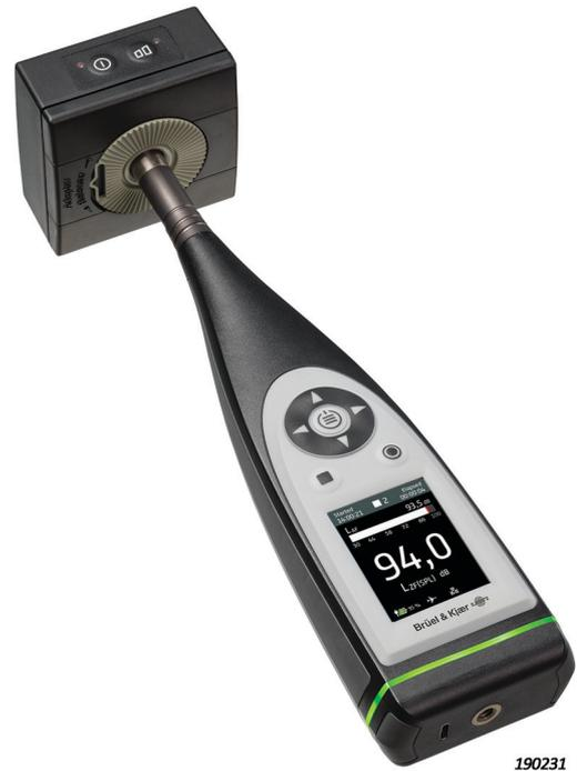
The calibrator gives a continuous sound pressure level when fitted on a microphone and activated.
