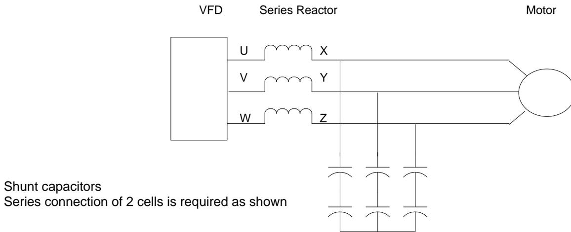
**NOTE: All 690V SWF filters require series connection of capacitors in each phase as shown.**
