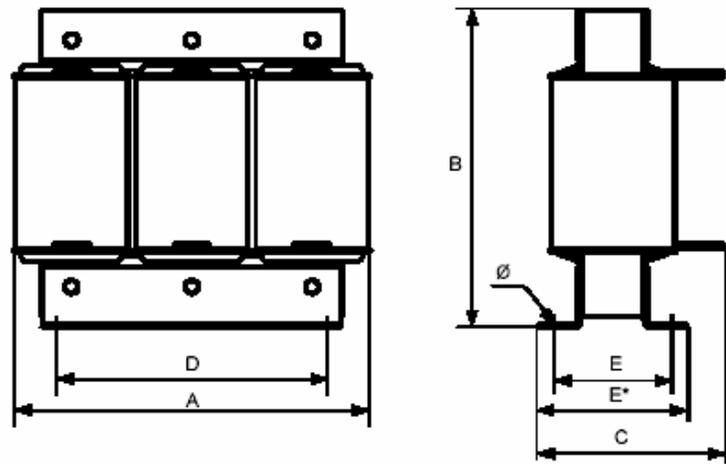
Series Reactor dimensions (inches) [Used for both 2.5KHZ and 5KHZ versions]
