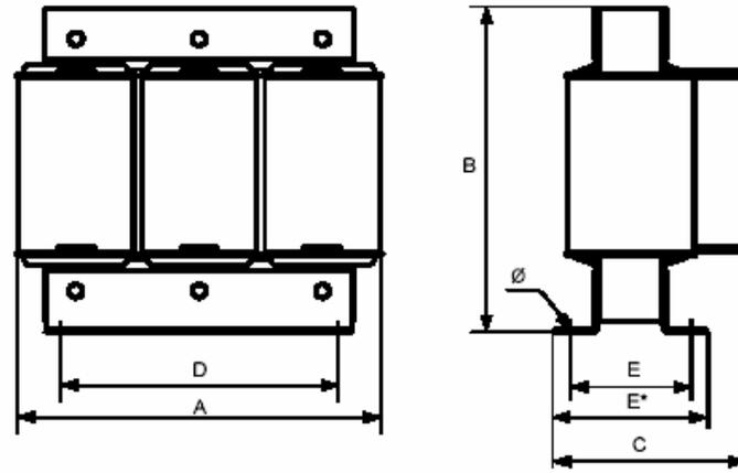
Shunt Reactor dimensions (inches) [Used in 2.5kHz version only]
